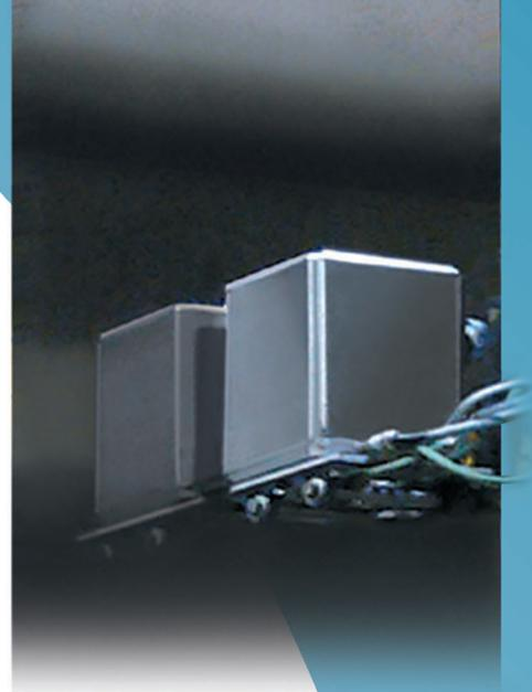
In hot-dip and electrolytic galvanizing lines the RS-40 X-ray fluorescence gauges are installed for non-contact, continuous and precise measurement of the coating thickness.
